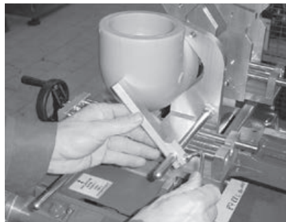
Fig. 7 Adjust the stop to hold the fittings
