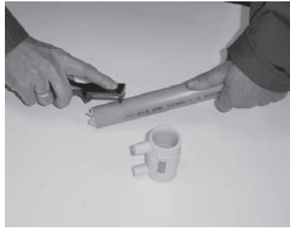
Fig. 2 Remove the outside oxide layer using a scraper.
