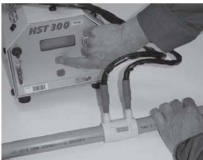
Fig. 7 Plug the cable plugs into the contact bushings. Enter the voltage and the welding time in the welding device. The welding data can be seen on the barcode label of the socket. Start the welding device with the switch.
