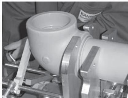
Fig. 11 Move the machine slides up to stroke end
