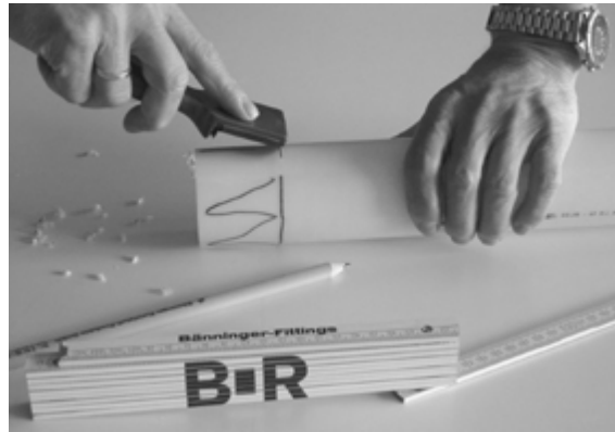
Machine the welding area surface with a draw blade Or a peeling tool in a shape cutting operation.
