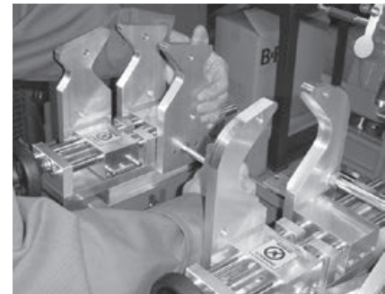
Fig. 3 Mount the prism clamping jaws
