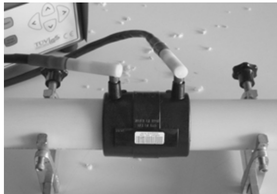
Connect the connection cables of the welding apparatus with the part to be welded. Fasten the welding cables in a weight-relieved manner.
